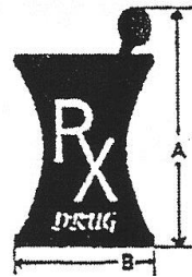
Display Area = area of Rectangle enclosing all Elements of the Display = "A" x "B"
